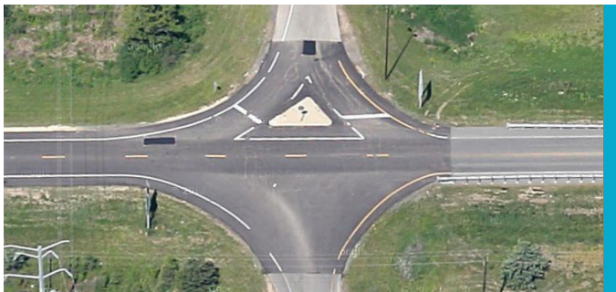
Figure 33. Utilizing Channelizing Island to Reduce the Exit Ramp Throat Width (Image: Google)
