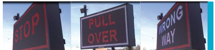
Figure 20. N.Y. Thruway Wrong-way Entry ITS Warning System (Images: taken from video from New York State Media Services Center)
