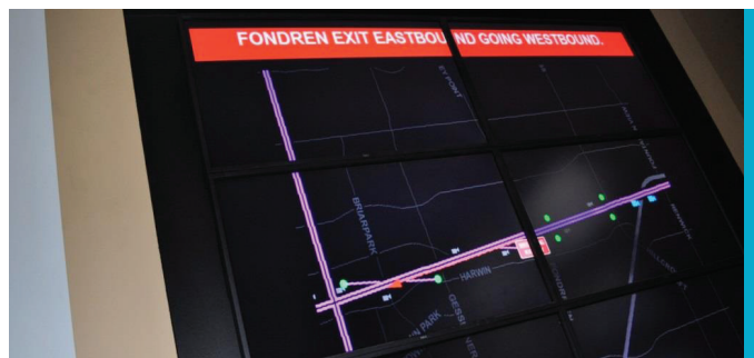
Figure 18. Automatic WWD Warning System at TMCs of the HCTRA (Image: Huaguo Zhou)
