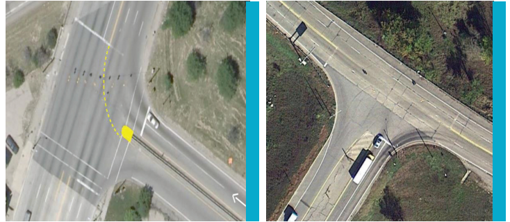
Figure 26. Pavement Marking Extensions for Left-turn Movement from Crossroad (left) and Stop Line (right) for Exit Ramps Next to Parallel Entrance Ramps (Image: MDOT)
