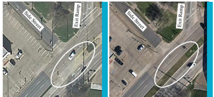
Figure 15. Before (left figure, 2009) and After (right figure, 2011) Pictures of the Modified Median at Wycliff Avenue (Image: Google Earth)
